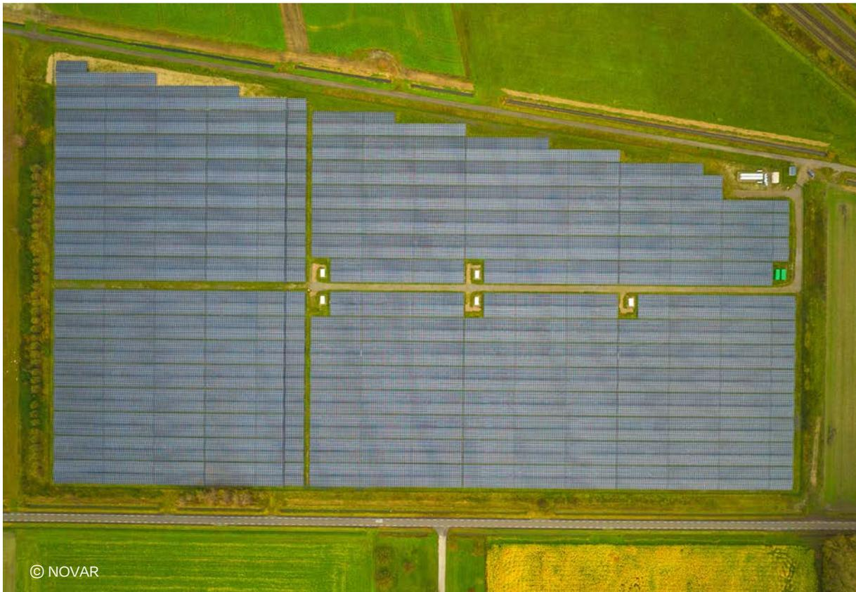
17.2 MW PV coupled with 5 MW / 5 MWh BESS, Bontepolder, the Netherlands
